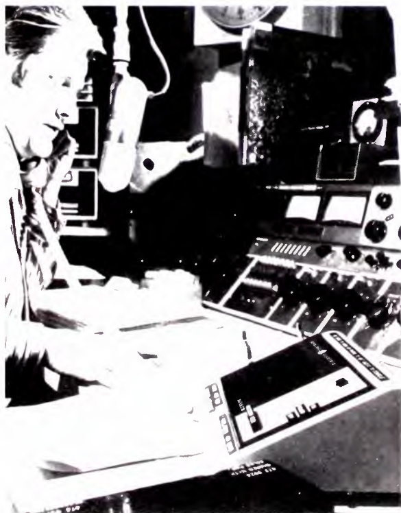
WHEN Radio's Jack Morse uses General Electric Deskon to his right in the control room to contact the airplane. When the studio is ready to have the traffic report broadcast to listeners, he "brings it in" through the console in front of him.
